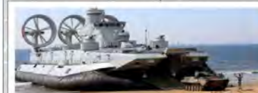
Zubr Hovercraft: Can quickly carry troops and light vehicles from ships to shore.
